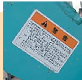
› Non-compliant example: warning on the boom in a non-EU language
