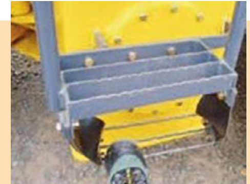
› This bottom step is too flexible (25 kg force should push the step inward by no more than 80 mm)
