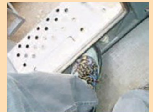
› This cabin has a tripping hazard on exit
