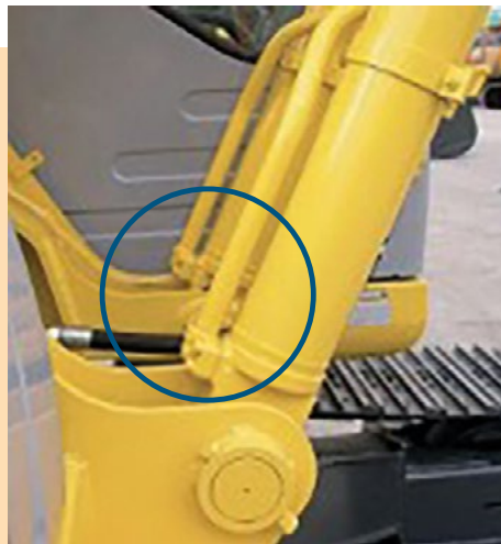
> This machine does not have lowering control devices. The pipes are connected directly to the boom cylinders
